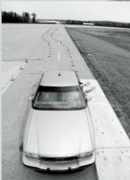
*Above and left, bird's eye view of precision docking. The Buicks consistently stopped at the "curb" with longitudinal accuracy of one foot, lateral accuracy of 5mm.*
