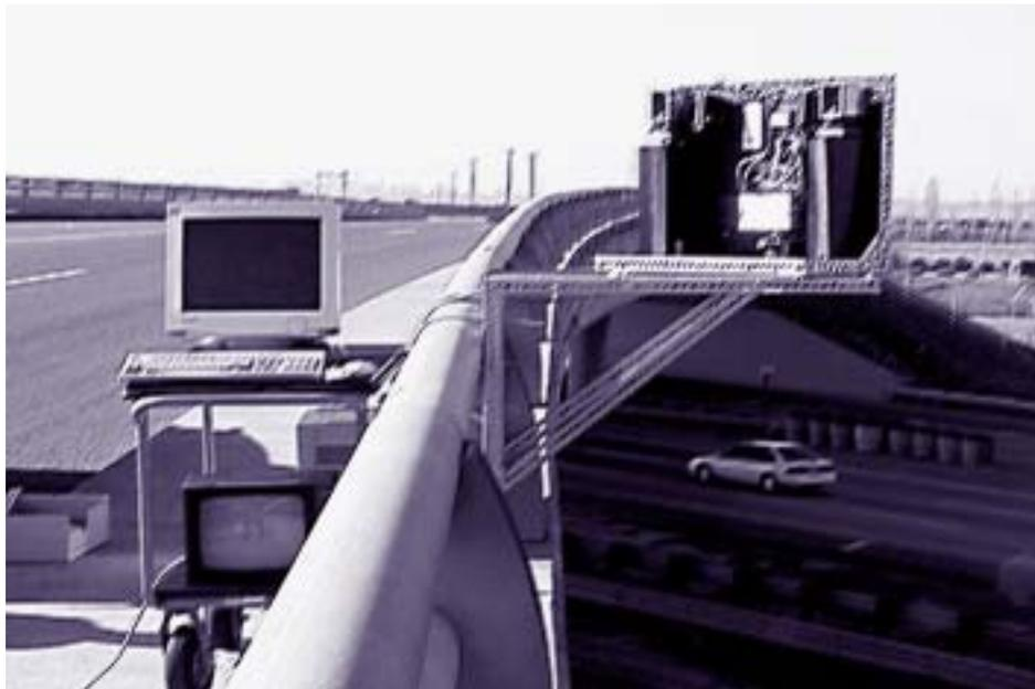
We have developed a new photodiode-array based system capable of measuring vehicles' speed and length that has several advantages over other systems currently in use. It is easier to install, more accurate, and requires much less computation, and
