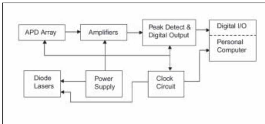
Figure 5. Block diagram of electronics hardware
