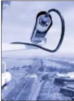
Figure 1. Berkeley Highway Laboratory surveillance cameras atop a 40-story building next to Interstate 80 in Emeryville provide ground truth for Caltrans loop detectors.
