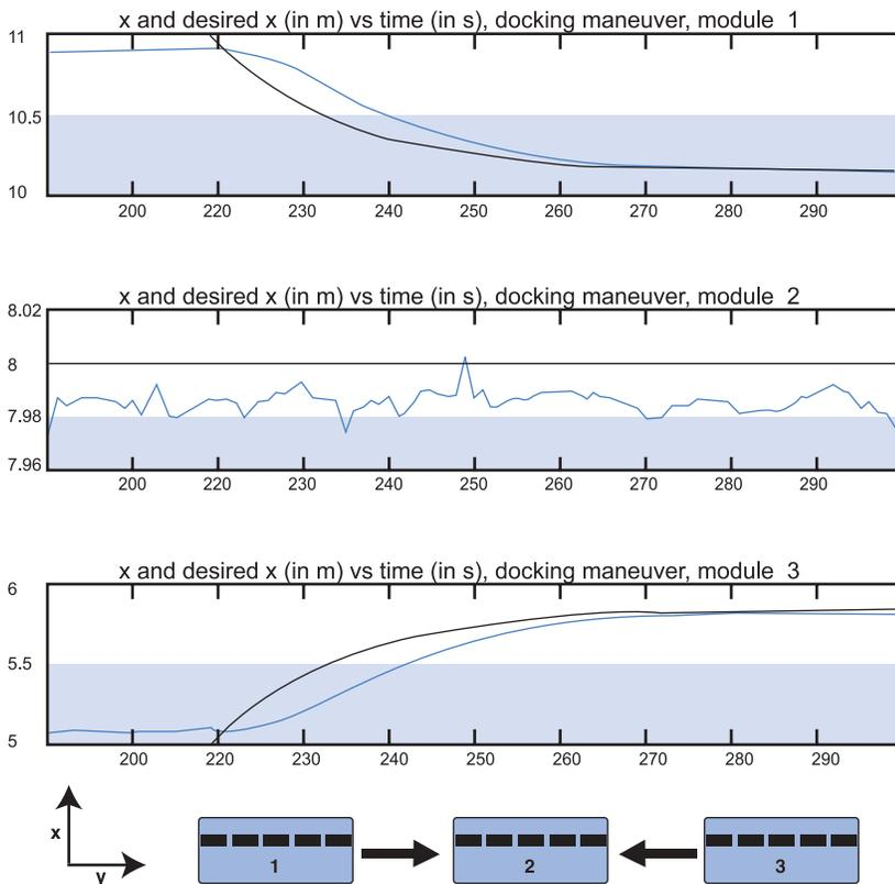
Figure 7. *x* position of the modules (in meters) vs. time (in seconds), while performing a precision docking maneuver. The desired positions are shown in blue and the actual positions in black.
