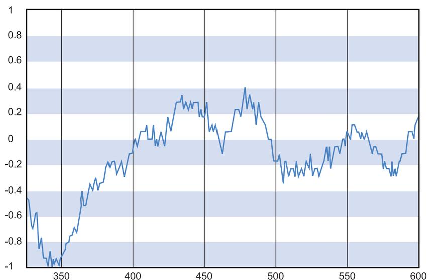
Figure 6. Heading angle of the module shown in figure 5 (in degrees), vs. time (in seconds), also while performing dynamic positioning. The angle is maintained within  $\pm 1$  degree of its desired value.
