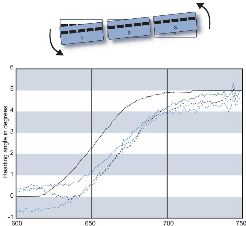
Figure 8. Heading angles of all three modules (in degrees) vs. time (in seconds) during a coordinated rotation maneuver from 0 to 5 degrees.
