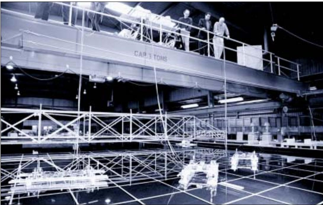
*Figure 4. Three modules are being operated from the bridge. The central computer is located on the bridge, and the umbilical cables that connect the central computer to the modules are visible on the picture. The umbilicals communicate power and control signals to the modules.*
