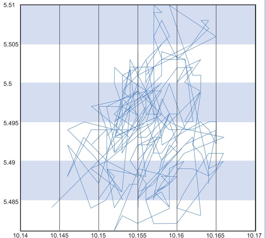
Figure 5. x position vs. y position of the center of gravity of one module while performing dynamic positioning at setpoint (10.15, 5.5).
