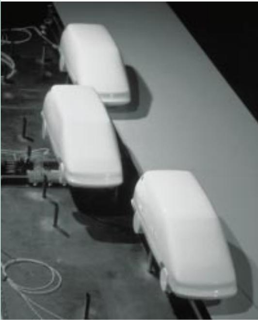
*Three-Lumina platoon in the Dryden wind tunnel at USC. A portion of the ground plane has been removed to show the support mechanism below.*
