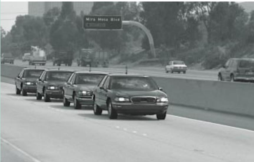
Test platoon operating at 4-meter spacing on limited access position of I-15 north of San Diego.
