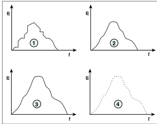
Figure 3 – Steps in vehicle signature feature extraction and data reduction process: 1. Full sample (actual data is discrete) 2. Low pass filtering and data smoothing 3. Amplitude normalization using wavelet transformation power spectrum and speed normalization 4. Data reduction
