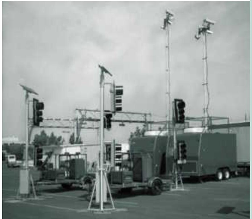
*Ramp-metering trailers with signal heads (front) and mobile surveillance trailers (rear)*
