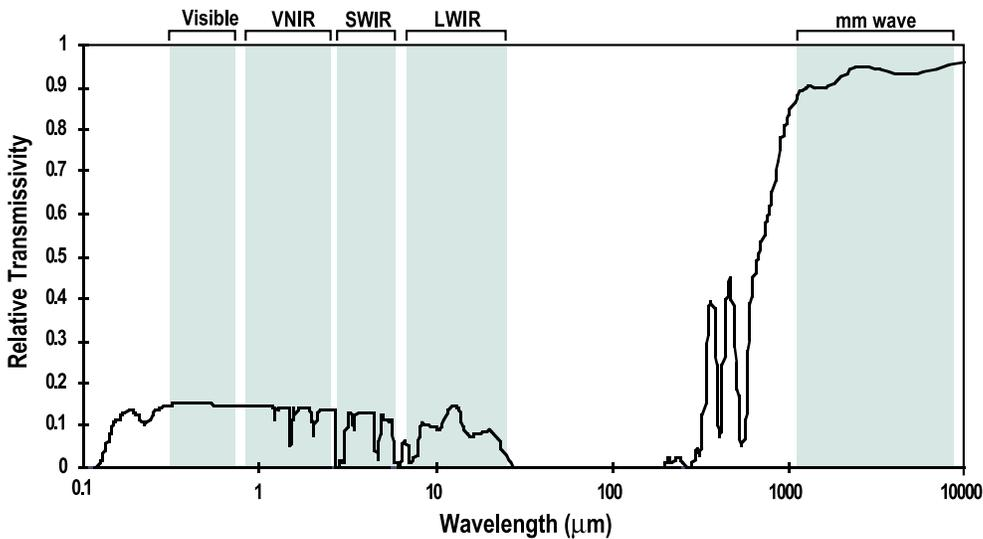
Figure 2 – Atmospheric Transmission, Medium Density Advective Fog
