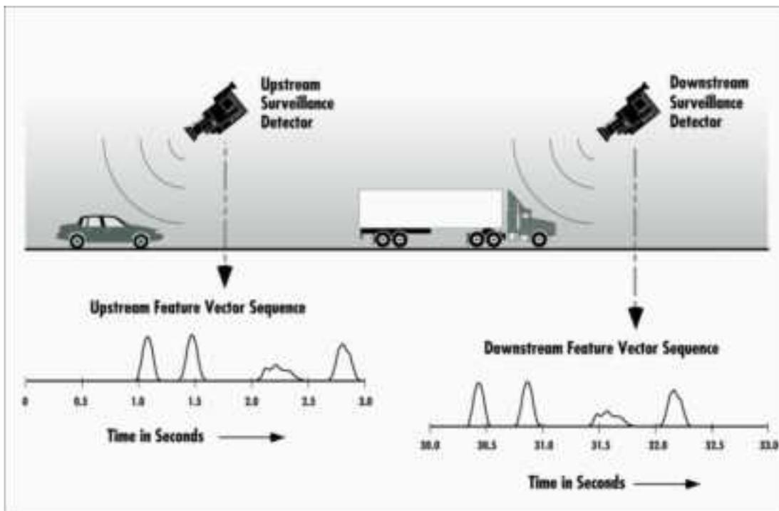
Figure 1 – Vehicle feature vectors are re-recognized downstream to general travel time. Dramatic changes in travel time indicates incidents. In this example, the platoon travel time is sequence offset (e.g. 30 sec.)
