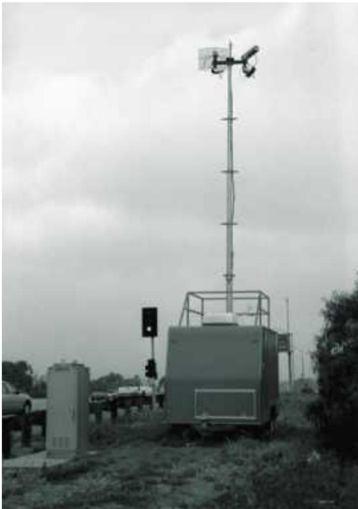
spread-spectrum radio link. The aggregated trailer data and one channel of video are also combined for simultaneous transmission to the Anaheim TMC and the UC Irvine Institute of Transportation Studies fixed sites
