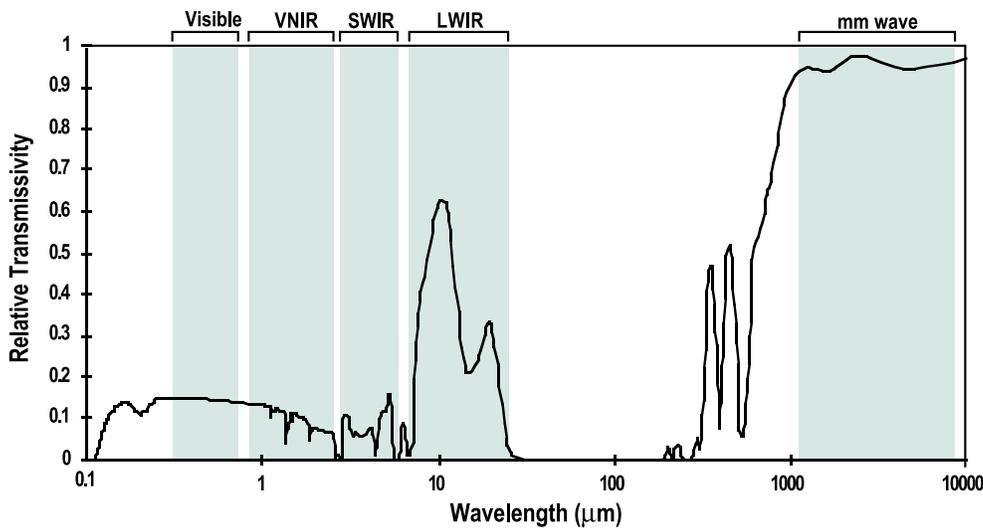
Figure 1 – Atmospheric Transmission, Medium Density Radiative Fog
