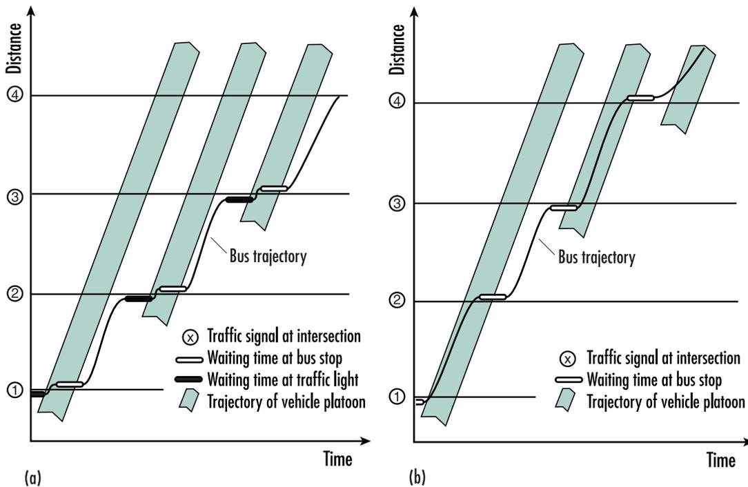
Figure 1. Trajectories of a vehicle platoon and a bus between successive signalized intersections. 1a—Bus stops at far side of intersections. 1b— Alternating near-side and far-side bus stops.
