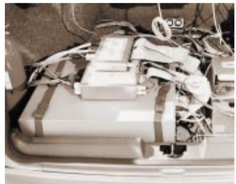
*Instrumentation, from top to bottom: Flux-gate magnetometer and ferrite magnet; Installation of magnets in roadway; Magnetometers mounted under bumper; Central processing computer and sensor interface boxes.*
