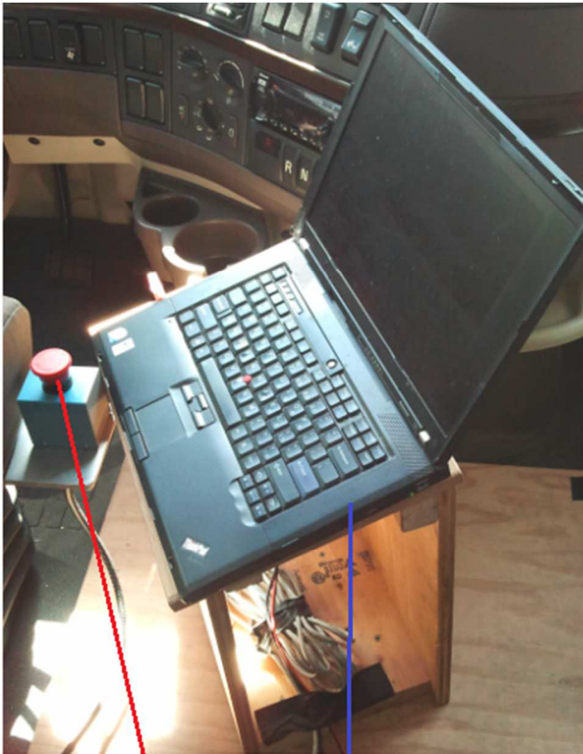
Emergency switch to cut-off link with J-Bus
