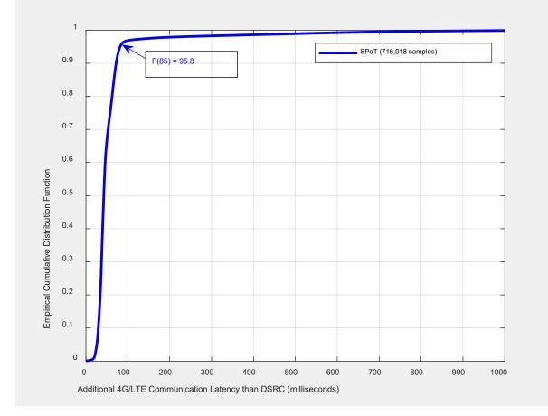
Communication latency difference = Message received time over 4G/LTE – (Same) Message received time over DSRC
