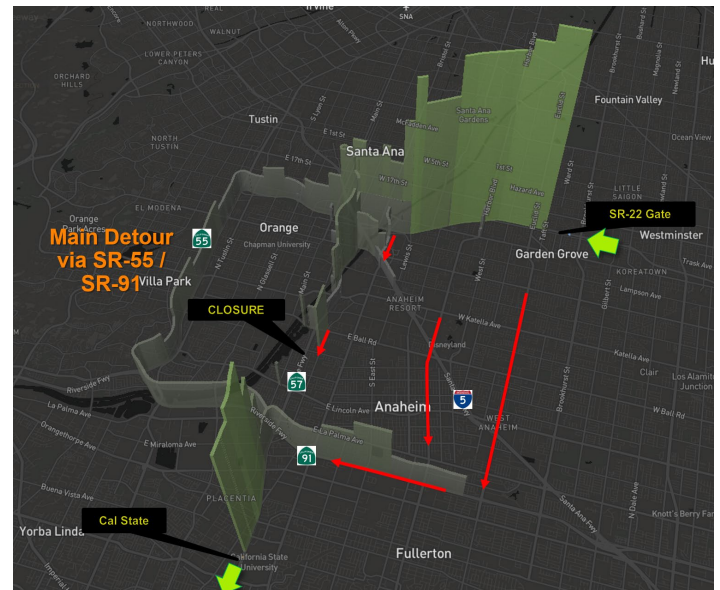
Figure 2: Streetlight top routes analysis from SR-22 to SR-57 near Cal State during a freeway closure of SR-57. The predominant detour on SR-55 resulted in substantially increased congestion on SR-55 on that day.
