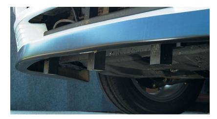
The magnetic field of magnets installed in the pavement is continuously monitored by a magnetometer array located at the vehicle front end. As the car passes directly over a magnetic marker, an onboard computer determines the marker's position relative to the array's center based on the measured magnetic field strengths and directions.
