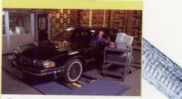
Faculty and students use the hemianechoic chamber at Ohio State's Center for Automotive Research to study automotive noise, vibration and harshness (NVH) control. The chamber is installed around a 150horsepower chassis roll dynomometer.
