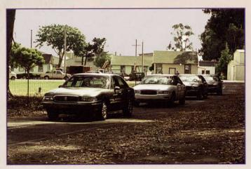
A line, or "platoon" of automated Buick LeSabres takes to the road at the Crow's Landing test site in preparation for Demo '97.
