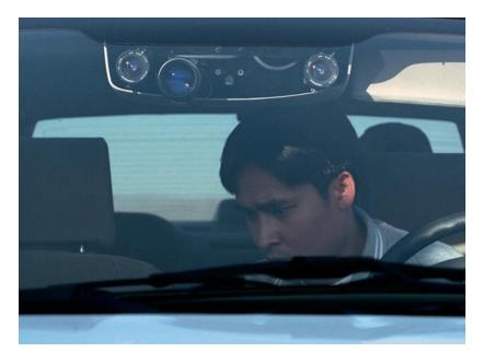
Stereovision cameras used in the Honda-PATH vehicles . The small cameras on the left and right are a stereo or binocular pair that allow the vehicle to see much like a person (the large camera is not currently used). A computer can compare the pictures from the two cameras and uses triangulation on objects in the image to determine the distance, which is useful for keeping a safe distance from the vehicle in front. (This system, still under development, is currently being tested.)
