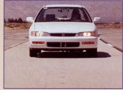
Front view of one of the Honda AHS Accords, which can drive using their own video cameras (visible through the windshield) or magnetized "nails" (shown here in the roadway).
