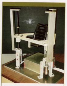
Driving simulators help researchers improve vehicle design and safety. Ohio State researchers built this quarter-scale tabletop simulator and are developing a full-scale model with a steering wheel, brakes and accelerator as a prototype for a commercial machine. The larger version will suggest the sensations of auto acceleration, deceleration and turning by tilting a person in the seat forward, backward and side-to-side.
