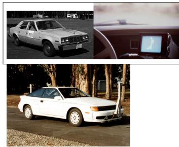
Fig. 3 First PATH Lateral Control Test Vehicles (AMC Hornet with magnetic guidance display and Toyota Celica with IMRA steering actuator and line-scan cameras for independent measurement verification)
