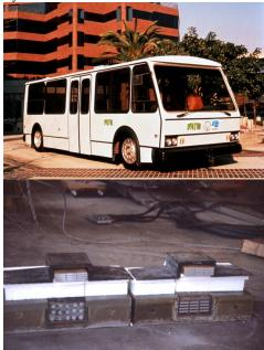
Fig. 2 Roadway-Powered Electric Bus and Cross-Section of Roadway and Onboard Power Inductors
