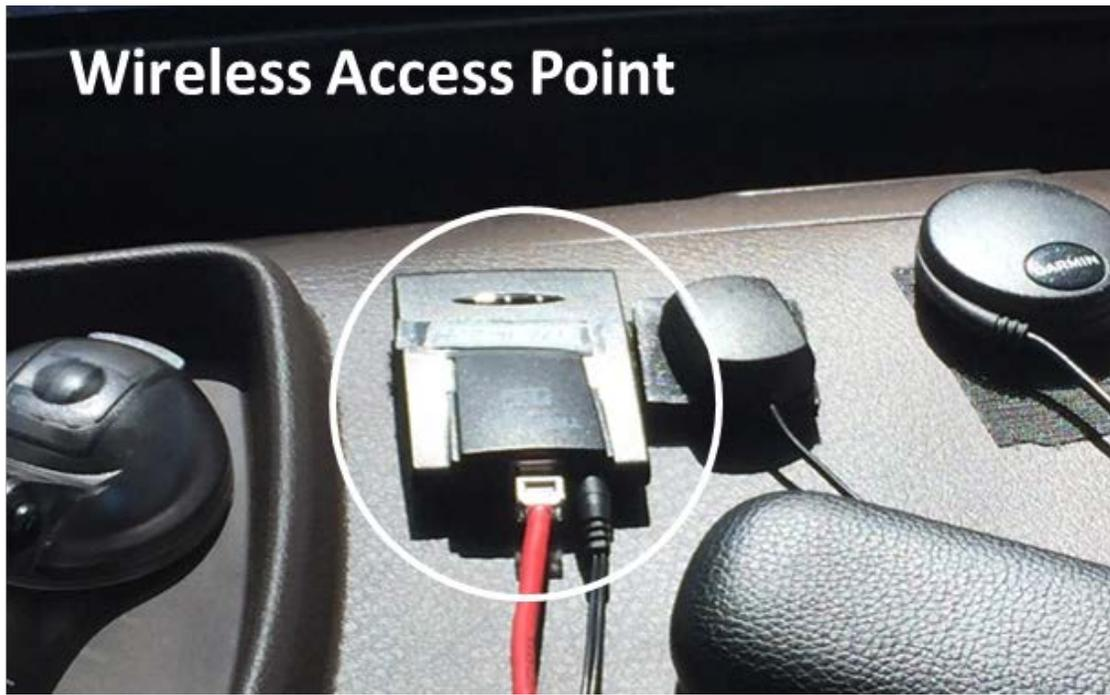
**Figure 6. Wireless access point on top of the truck control panel.**
