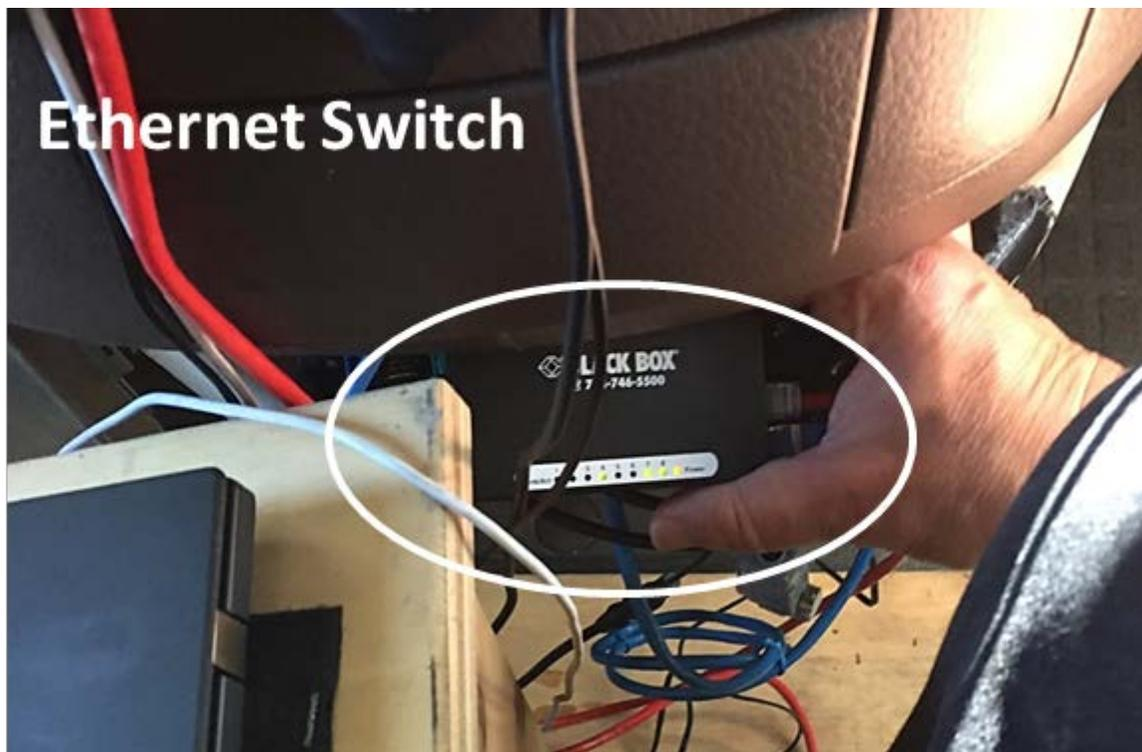
**Figure 8. Ethernet switch beneath the truck instrument panel.**
