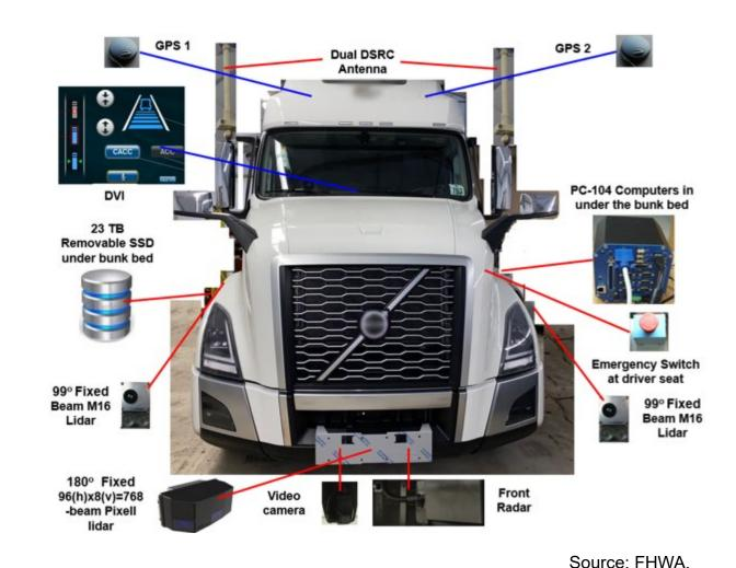
GPS = Global Positioning System; DVI = drive vehicle interface; SSD = solid state drive.
