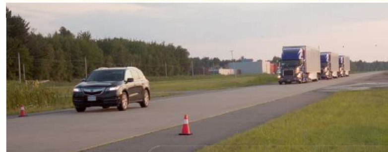
Manually driven SUV leading 3-truck CACC with 56m separation & 12m between trucks
