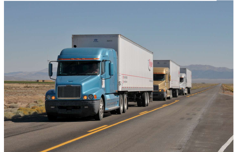
2009: 3-Truck Platooning with 4m on SR722 Nevada at 55mph
