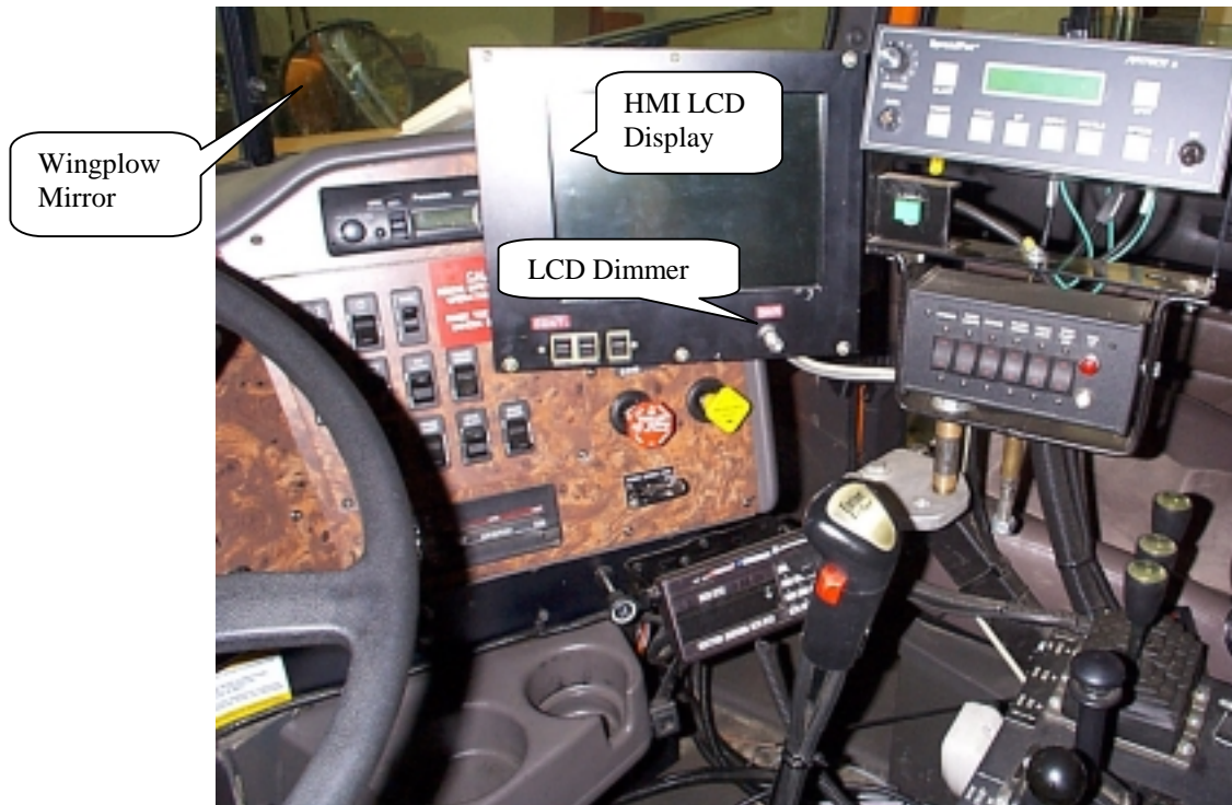
Figure 3-4: System Layout, Including LCD Panel for HMI
