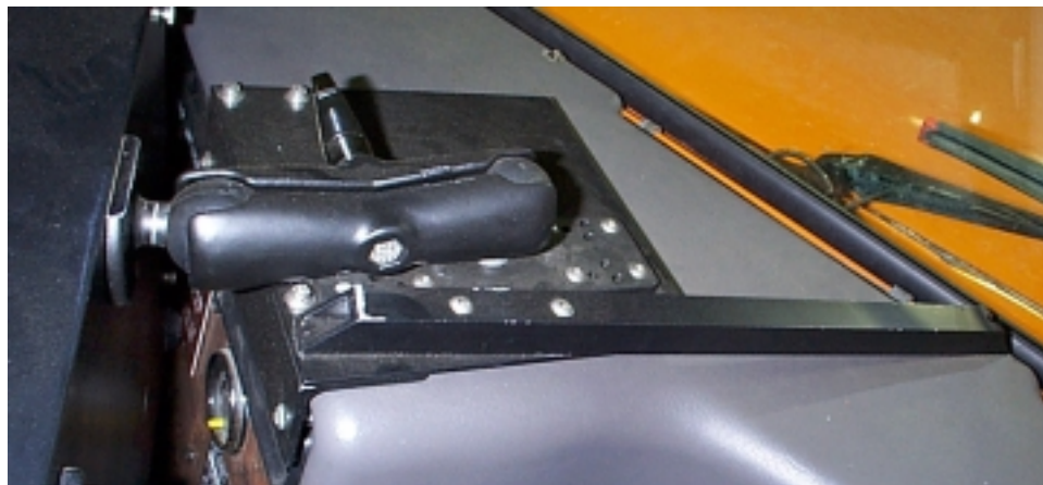
Figure 3-5: Hardware Mount for the LCD Panel
