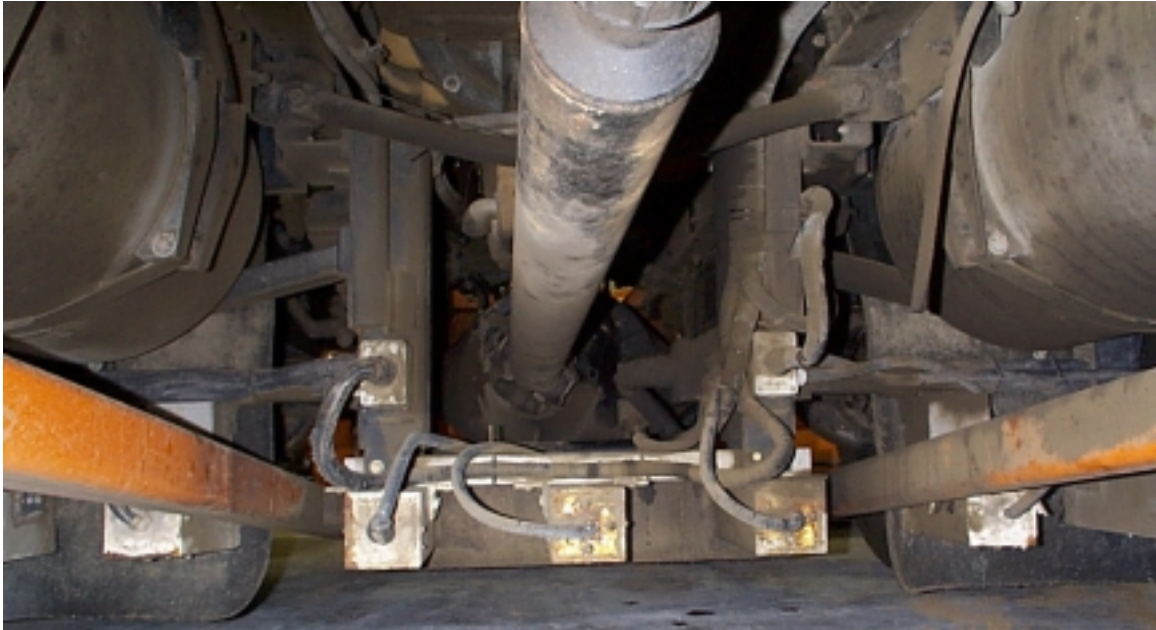
Figure 3-7: Center Portion of Front Magnetometer Sensor Array
