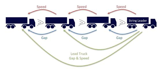
Figure 3.2. CACC Information Flow Post-Join Maneuver.
