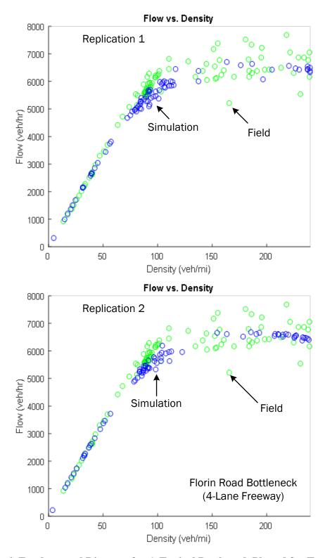
Figure 4. Fundamental Diagram for A Typical Bottleneck Plotted for Two Different Simulation Replications (Different random number sequences).
