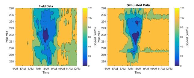
Figure 3. Field and Simulated Speed Contour Plots.
