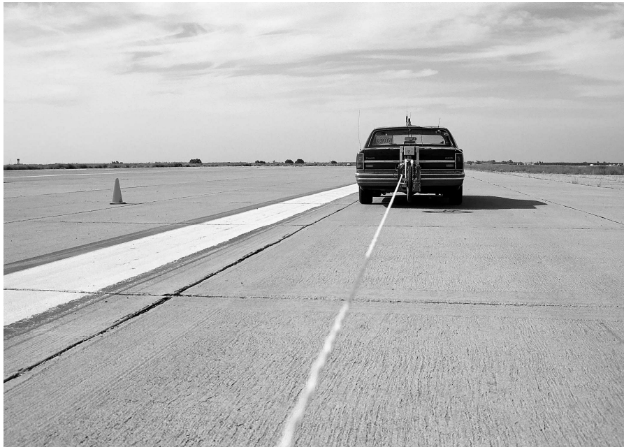
Figure 103 Using string port to detect true inter-vehicle distance on-the-fly
