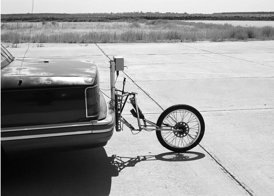
Figure 102 Fifth wheel to measure true ground speed and string pot (Top of the bar)
