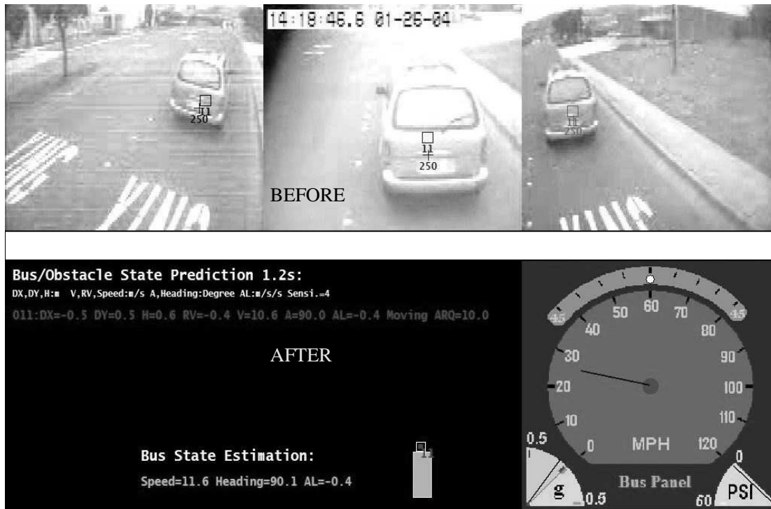
Figure 49 Following distance constraint (before and after)
