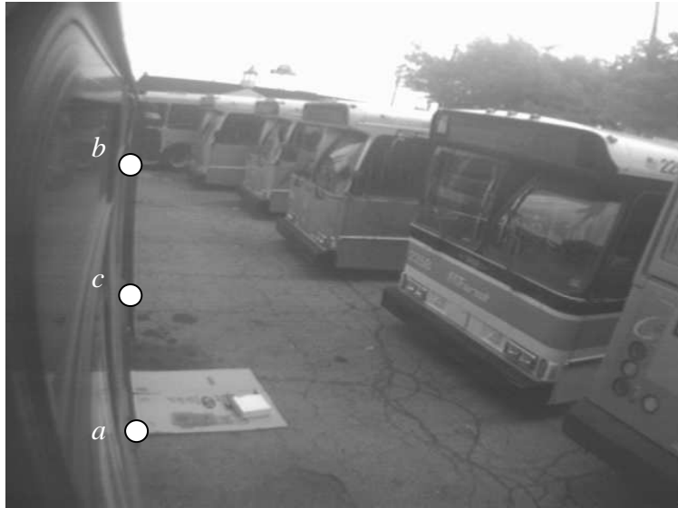
Figure 18 Example of three points chosen for the calibration. Point a is on the ground at the front wheel at the same y -position as the camera. Points b and c are edges at the lower and upper part of the open front door.
