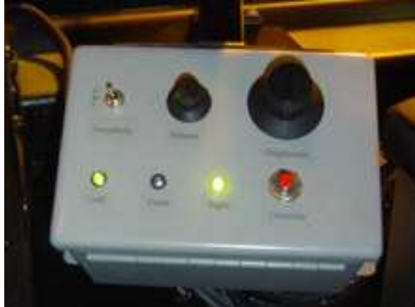
Figure 72 The DVI control box. The toggle sets the sensitivity, the knobs control volume and brightness, and the lights provide status information. Overrides are activated with the red button
