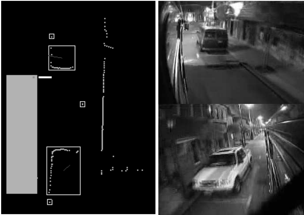
Figure 95 On the left side is a single laser scan segmented into different objects. The images on the right are from two video cameras and show the corresponding objects. Notice that the segmentation is not perfect, there are single points which are designated as separate objects even though they originate from the same car as a large object. The red line inside the large objects indicate their velocities.
