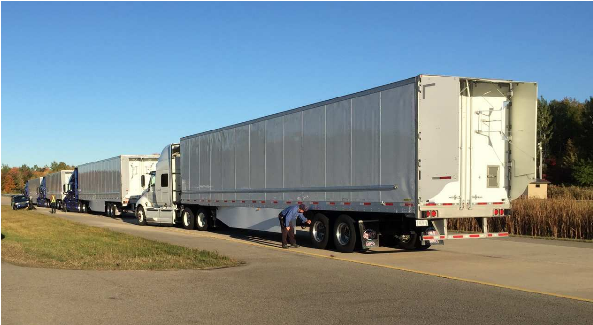
Figure 2.3: Test trucks 1, 2, 3, and the control truck parked in position on Bravo track during refuelling and tank weighing.
