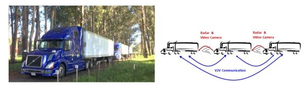
Figure 3. Volvo Class 8 trucks (left) and the V2V communication system (right).
