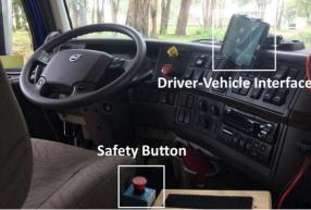
Figure 1. The CACC control stalk (left) and truck cockpit interior (right) with driver-vehicle interface (DVI) and safety button.
