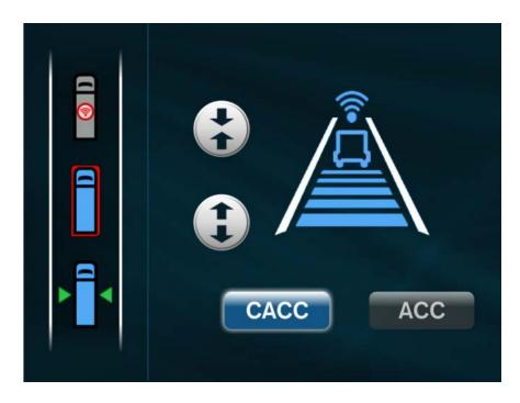
Figure 2. The display of driver-vehicle interface (DVI) inside the truck.
