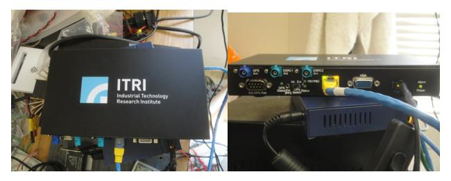
Figure 7. The top view (left) and side view (right) of DSRC radio.
