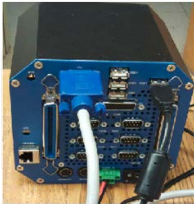
Figure 2-1 Assembled PC-104 and solid drive etc. with integrated CAN output interface port
