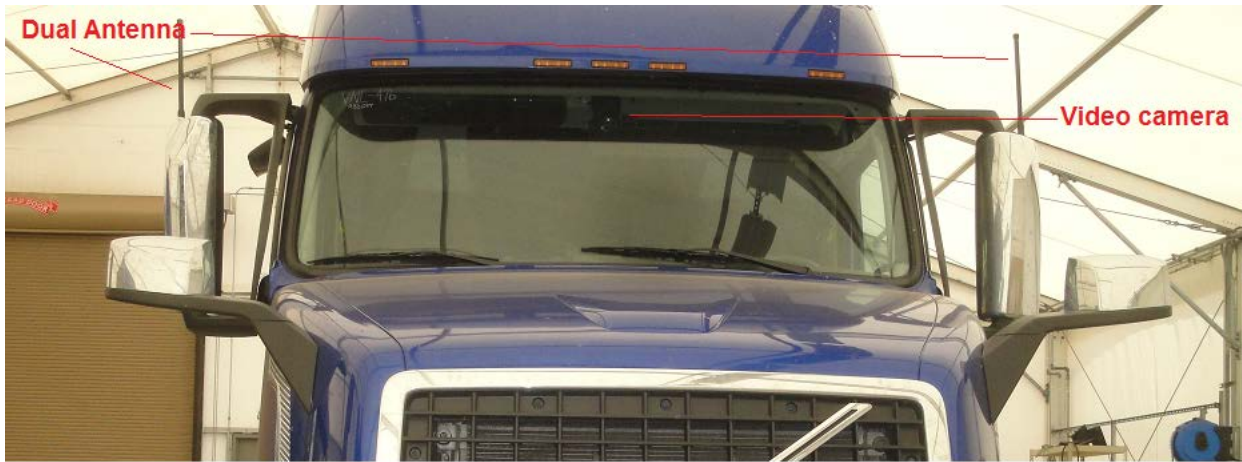
Figure 2-5. DSRC dual antenna installation on left and right mirrors.
