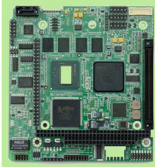
Figure 2-2. Intel Atom E640T CPU and Integrated Autocalibrating Data Acquisition
