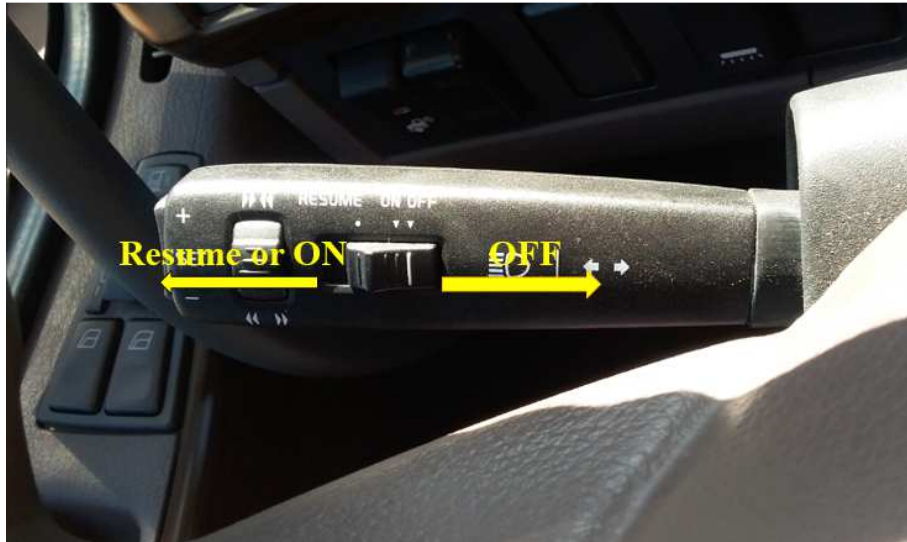
Figure 2-2. Automatic Control Activation
