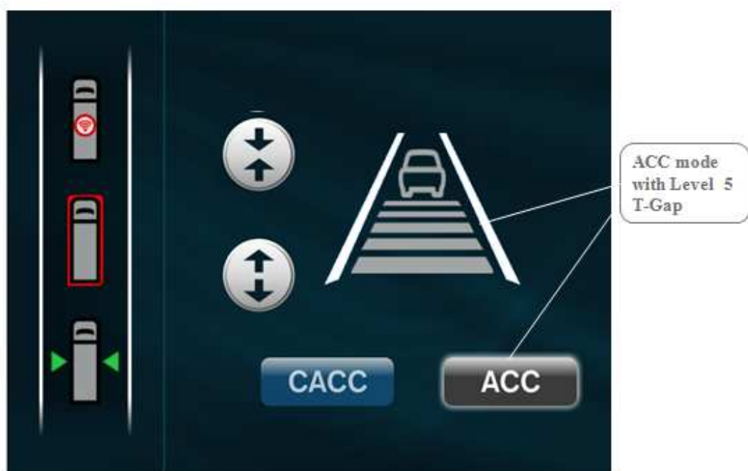
Figure 2-5. Driving Mode and Time Gap Selection: ACC
