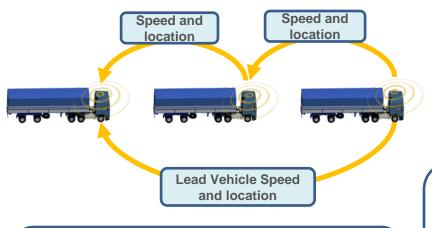
Benefits: The CACC system enables heavy trucks to safely drive in a closer than normal formation, with automatic control of their speed and spacing, while the drivers continue to control the steering and remain vigilant for any hazards in the driving environment. The close coordination of the CACC system has several advantages:
