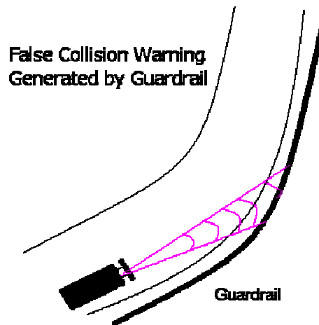
Figure 7-3: Diagram of Situation Capable of Generating a False Collision Warning
